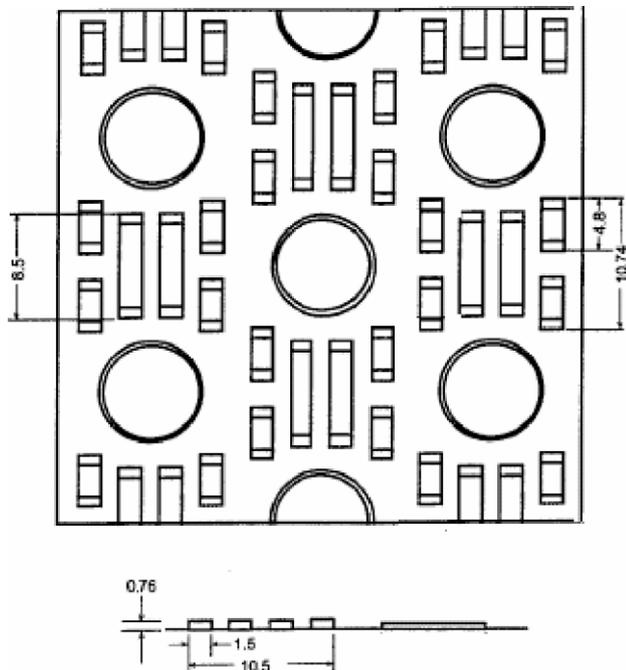
Fig. A.3. Geometry of slit-fin and round-tube heat exchanger.
