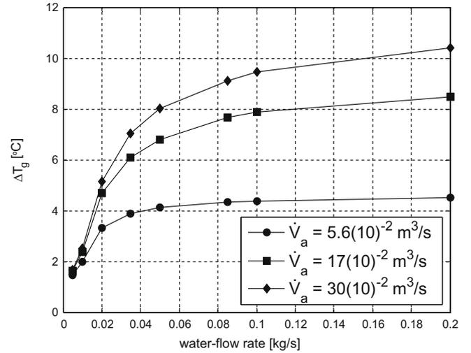
Fig. 10. Simulated results with various water-flow rates (curves shown for readability).
