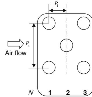
**Fig. A.2.** Geometric parameters related to tubes.
