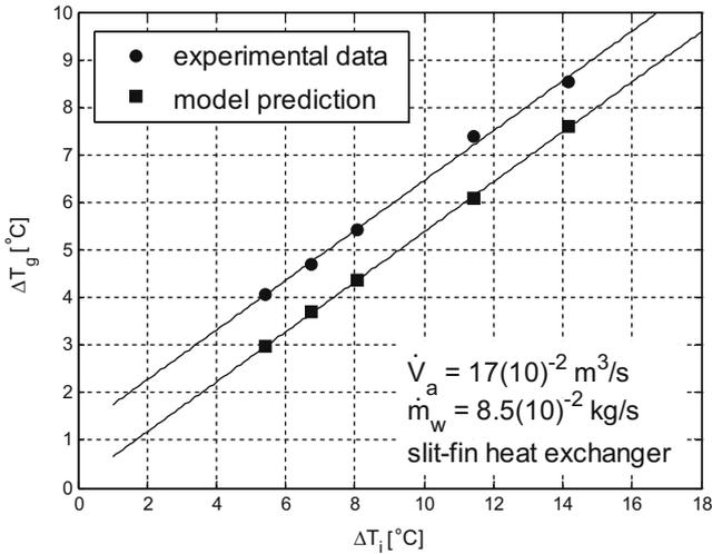
Fig. 8. Comparison of the simulation to experiments (slit-fin: lines shown for readability).
