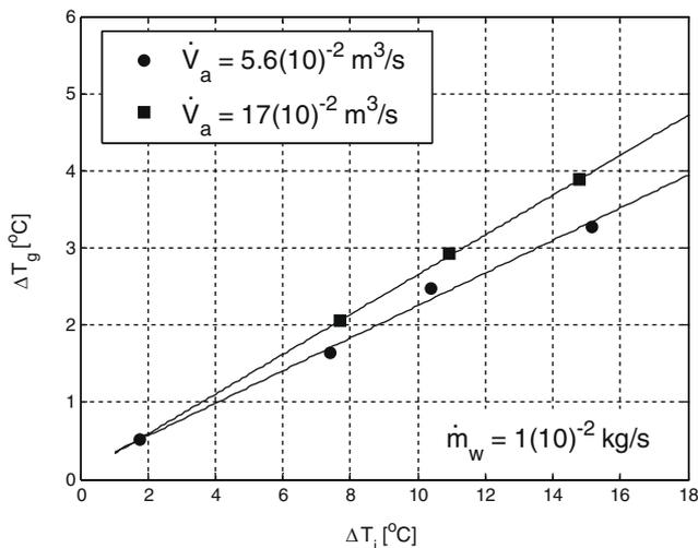
Fig. 4. Effect of air-flow rate (lines for readability).
