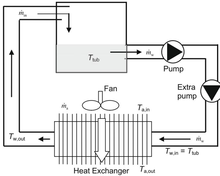
Fig. 2. System schematic of the simulation model.
