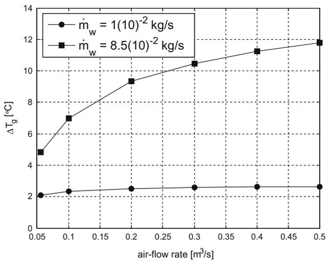
Fig. 9. Simulated results with various air-flow rates (curves shown for readability).
