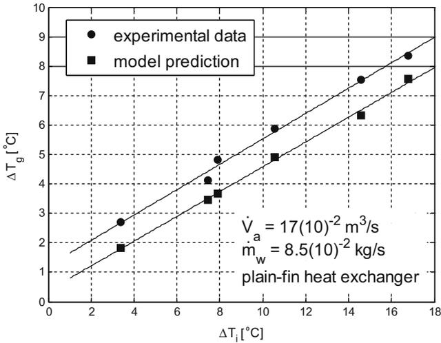
Fig. 7. Comparison of the simulation to experiments (plain-fin: lines shown for readability).
