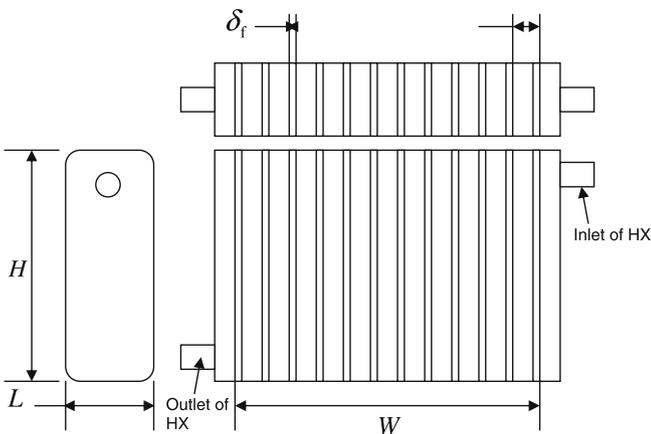
**Fig. A.1.** Geometry of plain-fin and round-tube heat exchanger.
