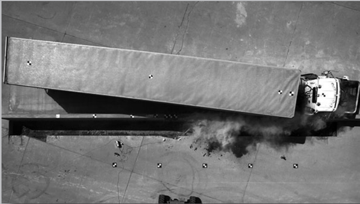
A shot from a video camera mounted on a crane shows an 80,000-pound tractor-trailer colliding with a concrete barrier during a test April 13 at the Midwest Roadside Safety Facility.
