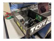
The purpose of this capstone project was to design and build timing circuitry to detect single photons. This project was designed in collaboration with the University of Nebraska Omaha physics department to measure fluorescent decay with sub-nanosecond precision. While our efforts to accurately detect single photons were not successful, the experimental enclosure was built, and the timing circuitry can accurately measure time delays between 14 nanoseconds and 500
